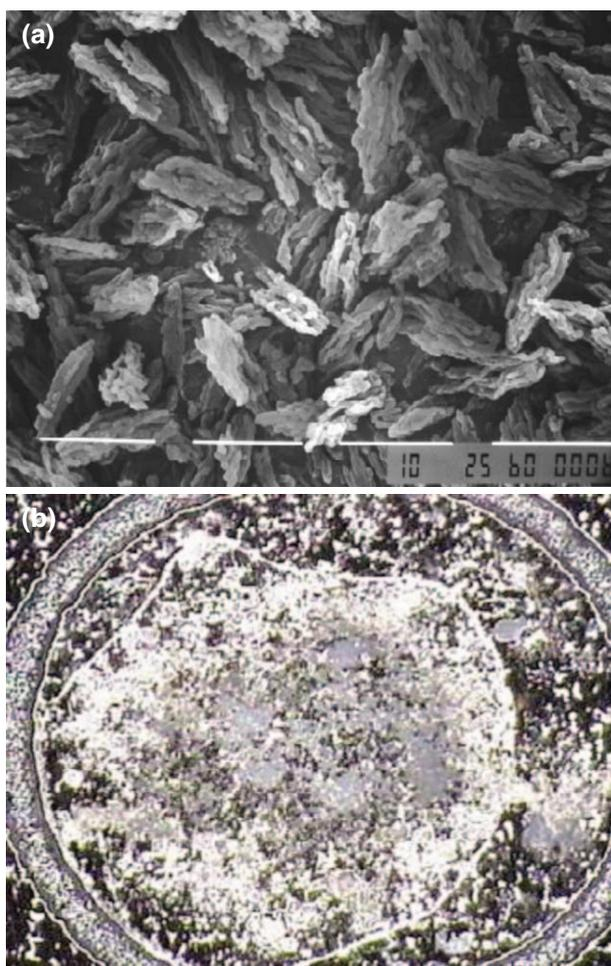
**Figure 1.** Image of deposited mesoporous silicate with sample on MALDI target plate. (a) SEM image of Al-SBA-15, (b) Photograph of deposited Al-SBA-15 with samples on MALDI target plate.
