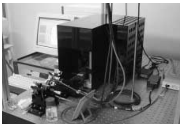
Figure 1. A self-developed spectral SPR biosensor.
